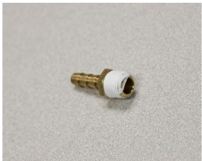
Figure 4: Incorrect Application of Thread Seal Tape
